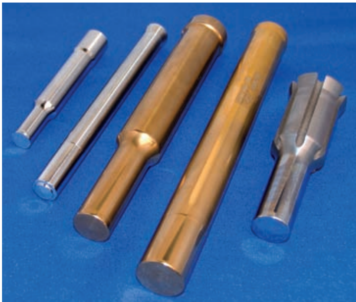
Hi-Quality Carbide grinds precision carbide punches that feature high length-to-diameter ratios. Punches range in size from 0.300"-dia. by 4" - long to 1.25"-dia. by 13"-long. They require a significant amount of precision contour grinding, must meet size tolerances of 0.000,3" – 0.000,5", and surface finish requirements of 2-3 \mu\text{m} . R_a prior to hand polishing.
